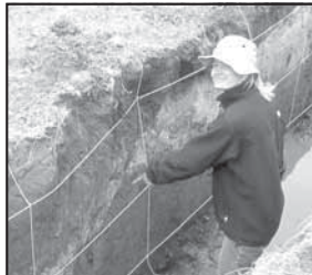
Scientists dig trenches across active faults to look for evidence of ancient earthquakes.
